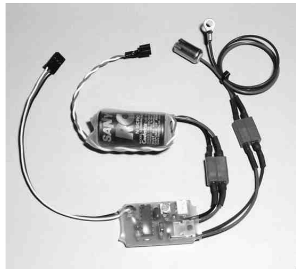
Figure 8 - A completed onboard glow system including the 1.2V NiCd battery and glow plug connector. This setup is illustrated with the original OPTOGLO design using a discrete MOSFET transistor.
