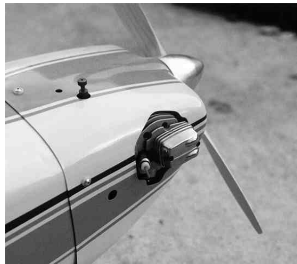
Figure 10 - Photograph of author's Pica 1/6 scale Cessna 182 with onboard glow connector in place.
