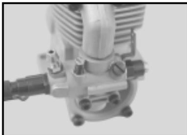
idle stop screw clockwise will make the throttle barrel stay open more. Turning it counter-clockwise will allow the throttle barrel to be closed more. Adjust the idle stop screw so that you can close the throttle barrel completely to shut off the engine. The rotor bolt holds the throttle barrel in the carburetor body and pre-
